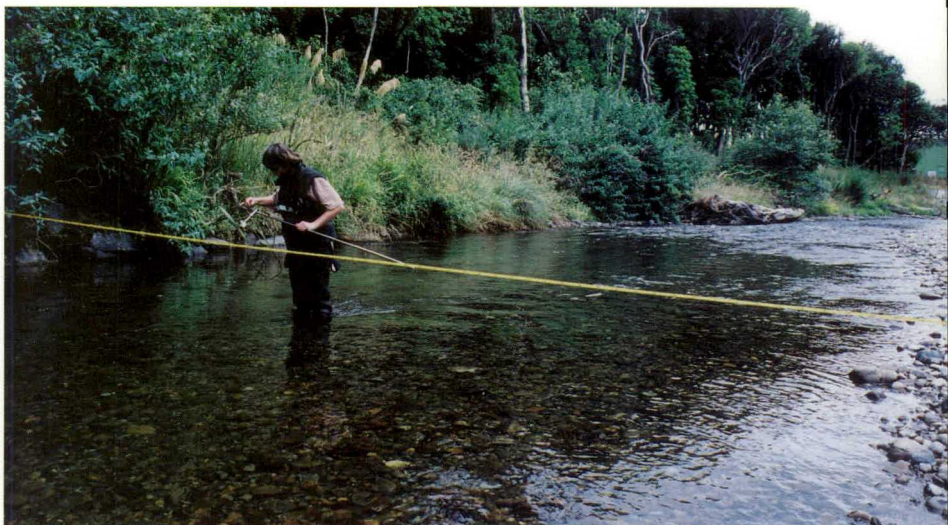
Greater Wellington staff measuring flows in the Waikanae River. We did this at about ten places along the river upstream from Waikanae to find out how much water was leaking between the river and groundwater. Both the river and the aquifer are used for water supply and we need to know the relationship between them so we can work out how much water it is safe to take.
