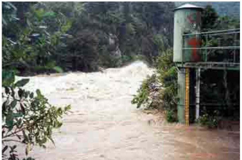
The flood of 28 October 1998 in the Hutt River. The green tower on the right of the picture is a river recording station – part of our flood warning network. Information on the height of the river is used by Greater Wellington staff to determine how big the flood will be further downstream in Upper Hutt and Lower Hutt.
