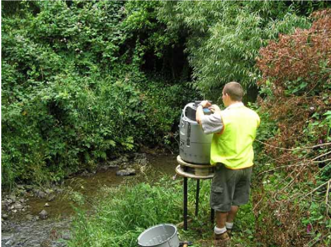
Figure 3.2 Setting up the automatic sampler in the Porirua Stream at No. 2 Tunnel (mid catchment) in December 2005
