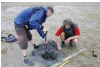
Burying sediment plates in the Porirua Harbour. The depth to each sediment plate will be measured each year, allowing us to determine the rate of sedimentation.
