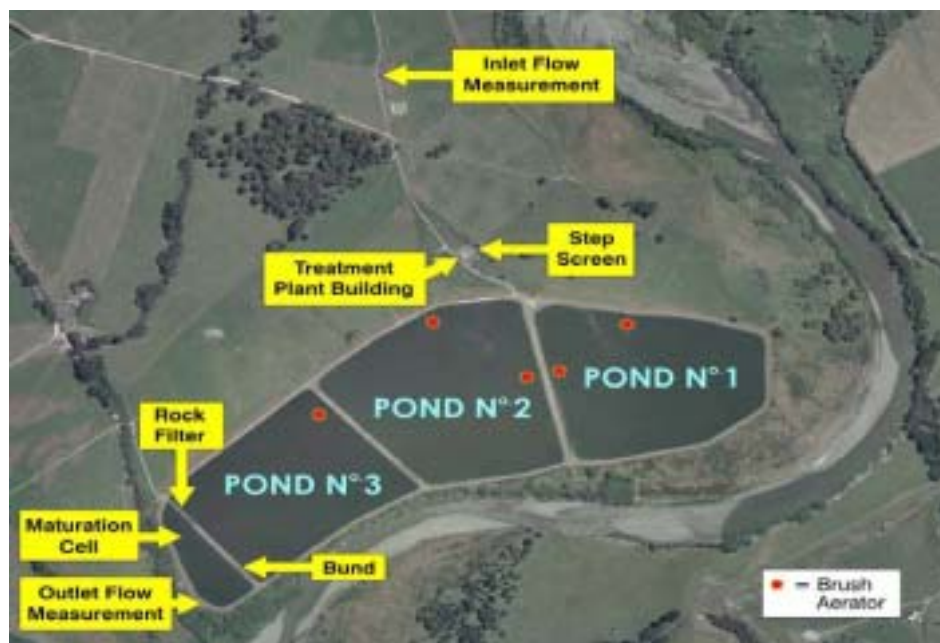
Figure 2 Key Components of Existing Treatment Plant
