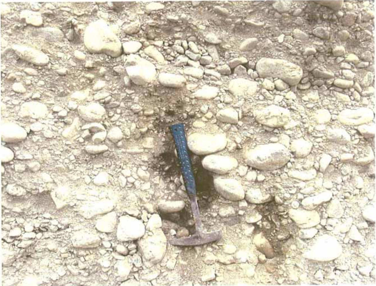
Figure 6: Typical In-Situ Profile of Gravel, Cobbles and Sand Forming Cut Slope in Old Excavation
