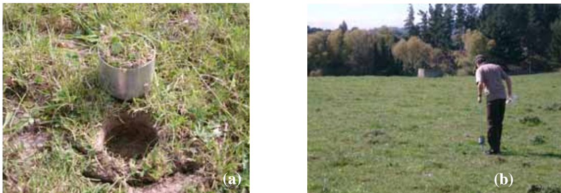
Figure 2.2: (a) One of three intact core samples taken at each site, to establish the physical properties of the soil. (b) Collecting a composite of core samples along a transect using a soil corer.
