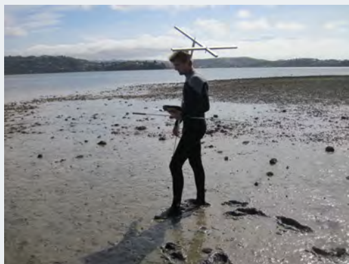
Measuring frame and probe used to measure shallow subtidal plates.
