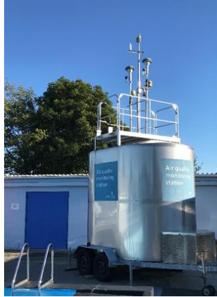
Mobile air quality monitoring trailer installed at Carterton public swimming pool measuring winter fine particle air pollution (PM2.5)
