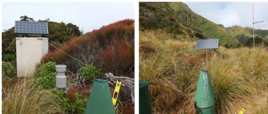
Tararua Range floodwarning rain gauge installations. Left: Mt Kapakapanui, elevation 1102m. Right: Penn Creek at McIntosh, elevation 1286m
