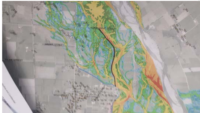
Figure 54: Investigation into possible alternative path for Western Stop Bank - design path in blue, alternative path in black
