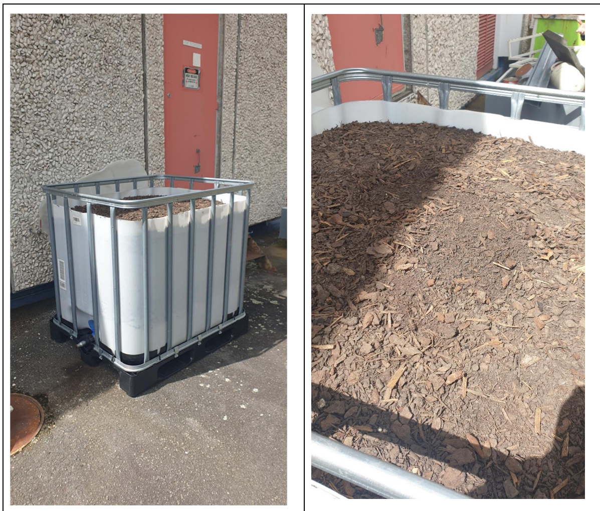
Figure 3.1: Pilot-scale biofilter (left) and close-up of media (right)
