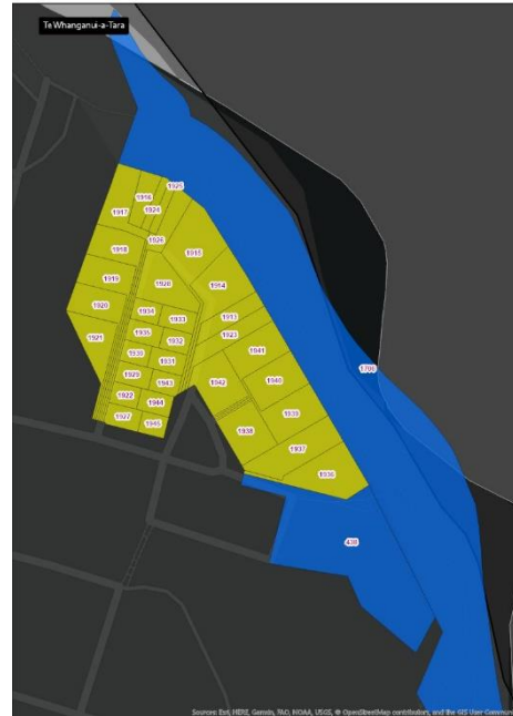
Figure 1.1: An example of an old landfill site that has since been subdivided into multiple residential lots. The yellow area on the left of the old landfill site has land that has been made safe for residential housing, while the blue area on the right still has contamination confirmed.
