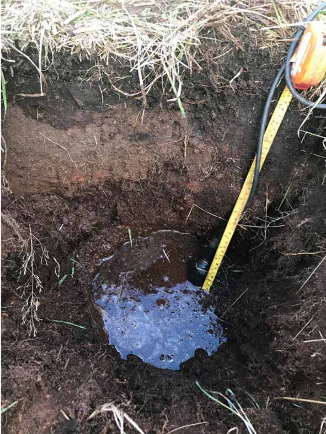
Figure A2.1: Peat Profile showing presence of water table and height of capillary rise
