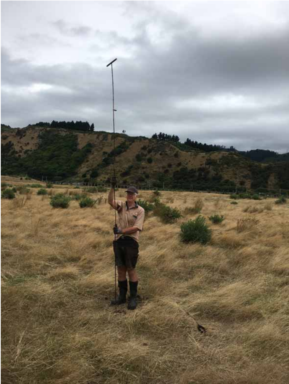
Figure A2.3: Probing survey underway. The depth of peat at this site is indicated by position of clothes-peg attached to upper section of probe.
