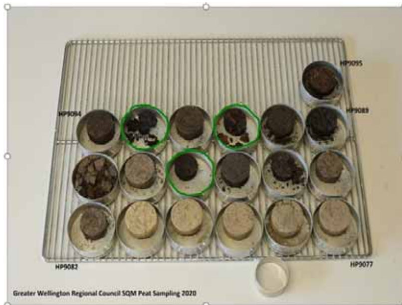
Figure 4.6: Soil cores from 2020 sampling – the ring in the foreground indicates the original volume of soil
