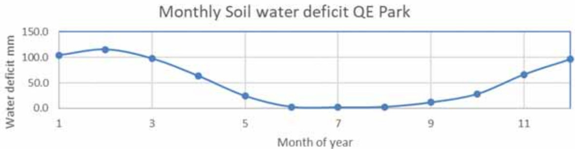
Figure 4.7: Monthly average Soil water deficit QE Park based on 150 mm storage in 0-600 mm depth range
