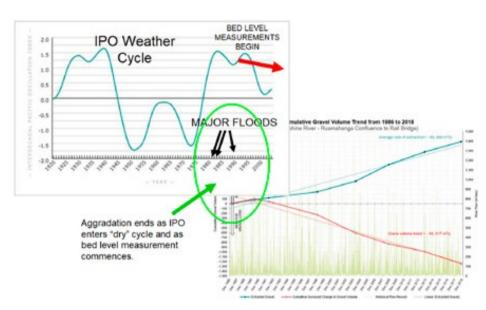
Figure 29: IPO "Dry" cycle begins as bed degradation and measurement begin.
