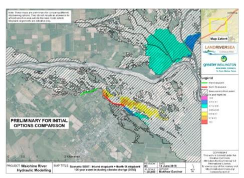
Figure 45: Shows minimal change in flood depth due to inland stopbanks and shows urban area saved from flooding.
