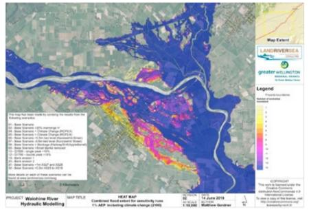
Figure 36: Significant flood sensitivity scenarios laid one on top of another to see maximum extent - landriversea Consulting.
