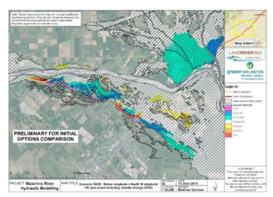
Figure 48: Option 3 North St Stopbank plus Greytown Stopbank Extension to XS 30 – landriversea Consulting.
