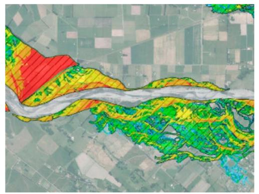
Figure 65: Attempt to force extra flood water at end of Greytown Stopbank (+20% bed roughness on top of 1:100 year plus climate change) makes little difference but has some negative downstream effects.
