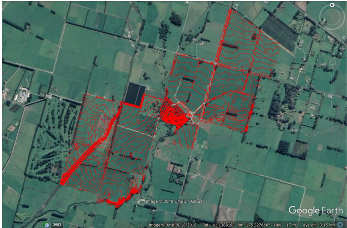
Figure 1 Raw Drone Survey Showing 30 cm Contours
