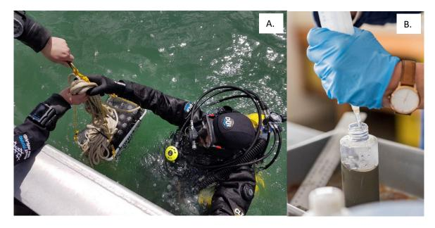
**Figure 2-3: Examples of sediment cores collected from Wellington Harbour.** A. Crate of sediment cores being transported to the boat by diver after collection (photo: Peter Marriott, NIWA); B. Seawater being carefully syringed off the core surface prior to extrusion and sectioning (photo: Dave Allen, NIWA). Only the top 30 mm of sediment was collected for sediment chemistry and particle size analyses.
