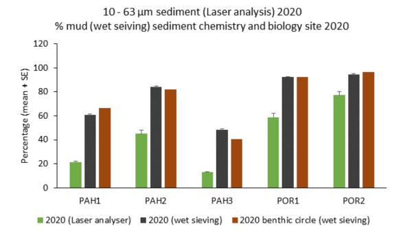
**Figure 3-9:** Concentration of finer sediments in 2020 determined using laser analysis and wet sieving. Plot shows the percentage of 10-63 Im sediments determined from the sediment circle using the laser analyser (N=3; green bars), and of mud sized particles (0-63 Im) using wet sieving analysis (N=3; black bars). Also shown are the percentage of mud from the benthic circle (N=1; brown bars).
