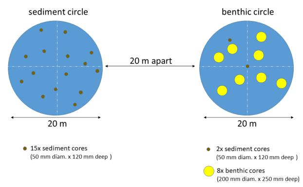
Figure 2-2: Schematic of subtidal sampling methodology followed for collection of sediment chemistry and benthic faunal samples from Porirua Harbour in 2020. Not to scale.
