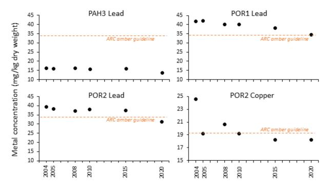
**Figure 3-10:** Concentrations of metals over time. Only metals and sites for which statistically significant correlations were detected are presented.
