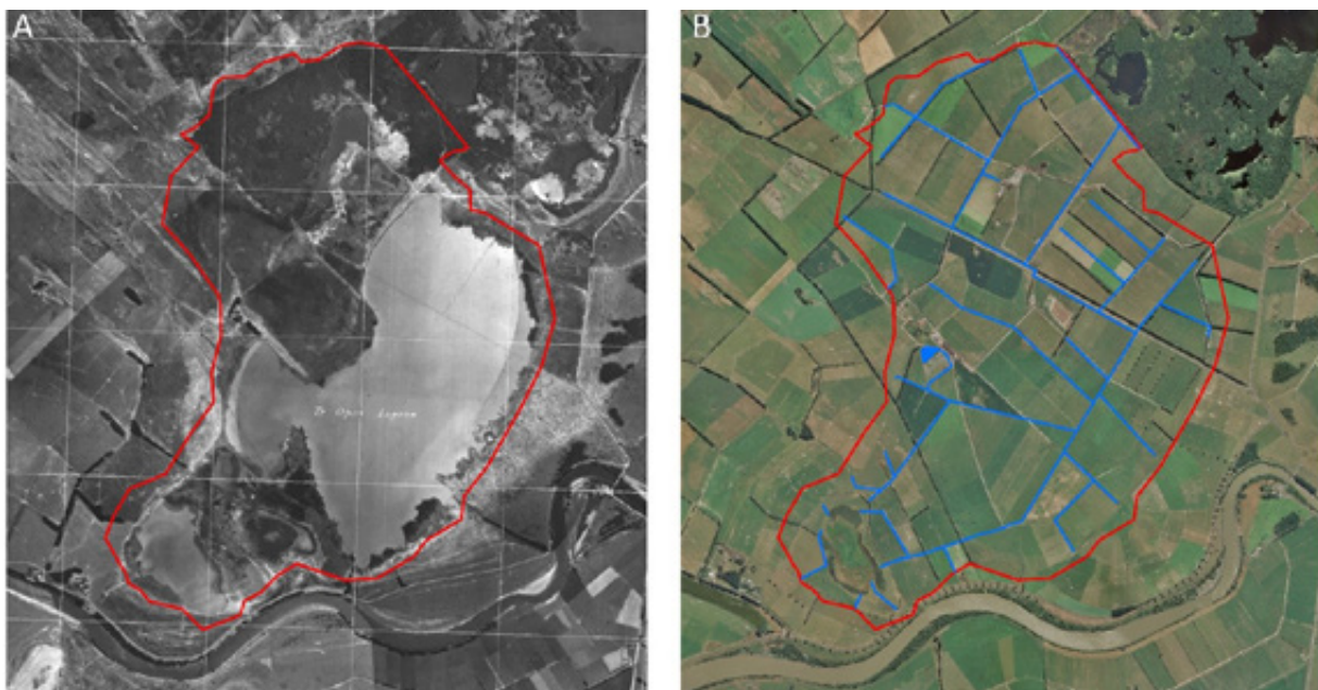
Figure 1: A) Aerial photograph taken in 1961 depicting the historic (pre-drainage) extent of open water in the Te Opai Lagoon area near Lake Wairarapa. B) Aerial photograph of the Te Opai Lagoon area post drainage (2017). The blue lines represent the highly modified streams.
