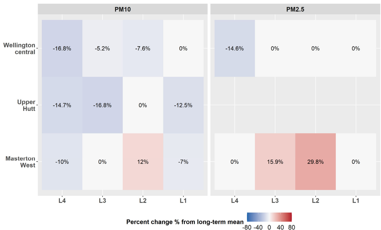
Figure 4.14: Percentage difference 7 between observed PM and long-term (2016 to 2019) mean across all three sites by Alert Level. Where the percentage difference was not different from zero at the 95% confidence level, the percentage difference is shown as 0%.
