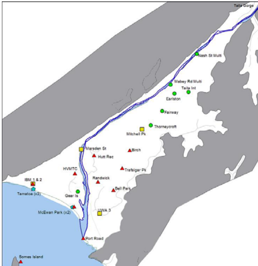
Figure 5.6: Locations of groundwater level monitoring sites in Lower Hutt. Green circles – Taita Alluvium; yellow squares – Moera Gravels; red triangles – Upper Waiwhetu Aquifer; blue hexagons – Lower Waiwhetu Aquifer.
