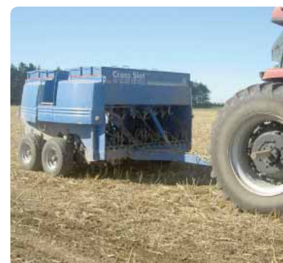
Cross Slot drill being used to establish wheat directly into brassica residues
