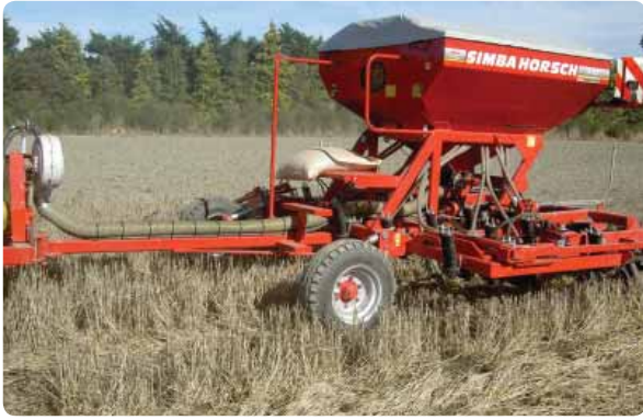
Four metre Simba Horsch CO4 band coulters drill sowing direct into chopped wheat straw - autumn sown second wheat
