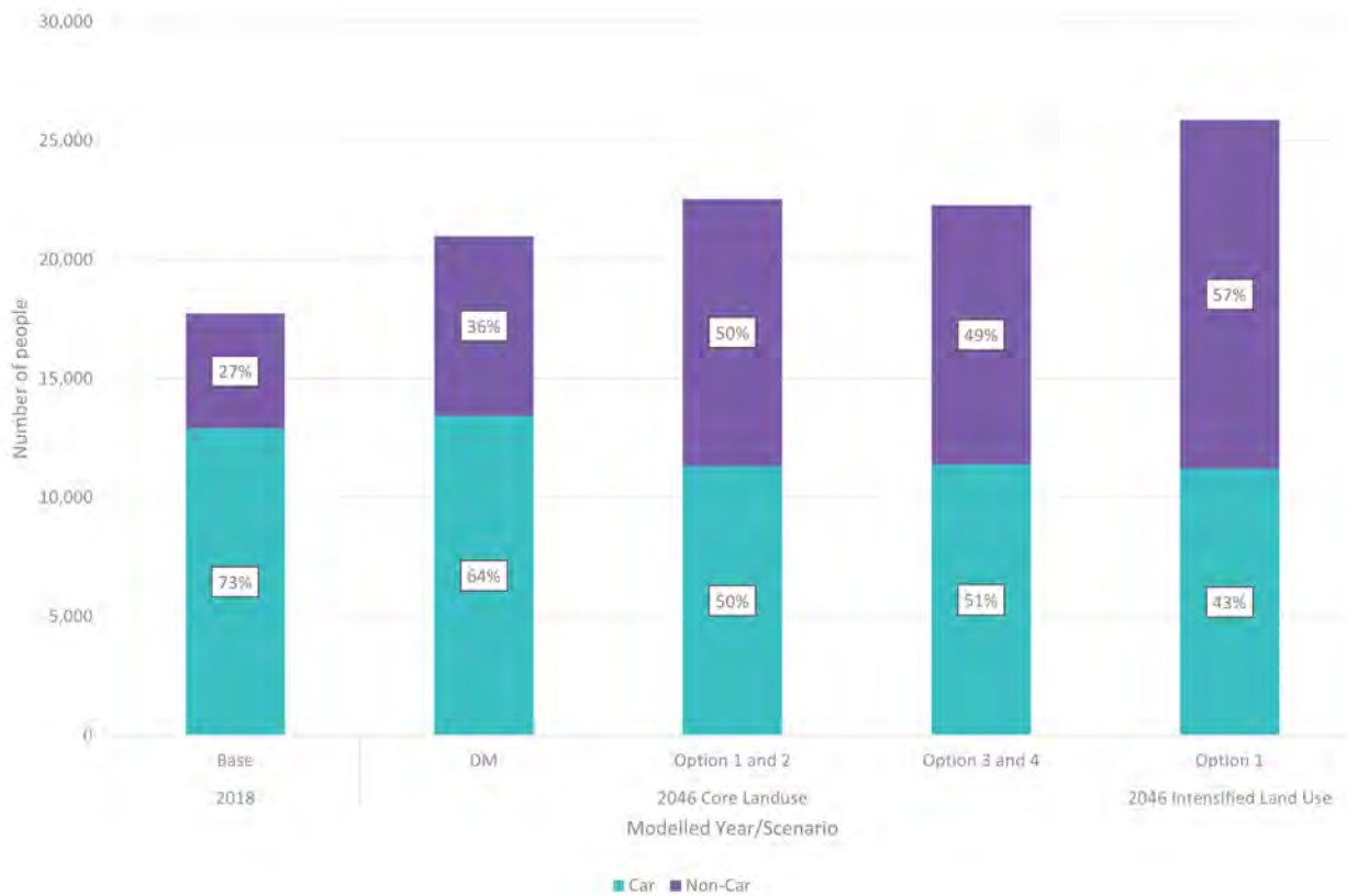
Figure 11: Car and non-car mode share, AM peak, traveling to CBD from south and east suburbs (WTSM April 2022 preferred option modelling)
