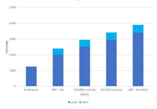
Figure 12: Southern corridor PT line loading 2046, inbound AM peak (preferred option modelling WTSM, 1-hr volumes at peak loading point – approaching BR)
