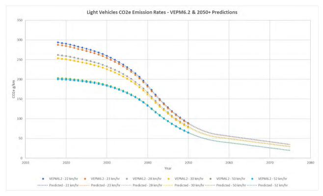
Figure 7: Carbon emissions rates - VEPM and 2050+ predictions
