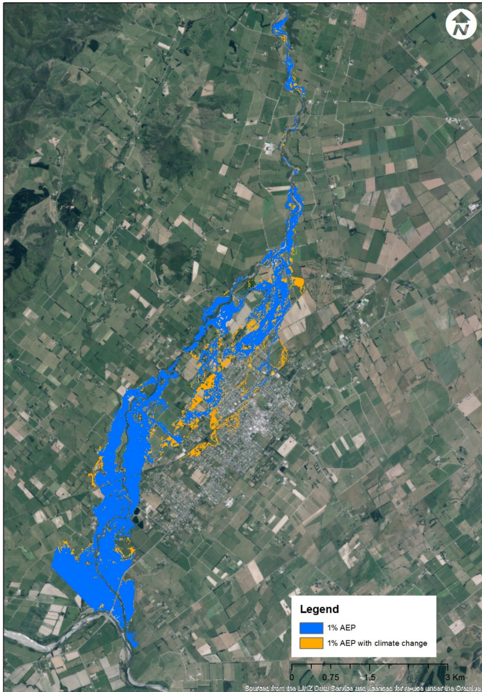
Figure 5-2: Differences between modelled flood extents predicted as a result of 1% AEP flow and a 1% AEP flow with an allowance for climate change
