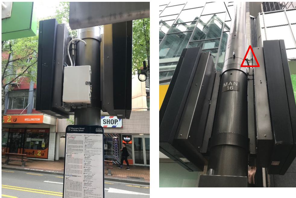
Figure 4.2: Enclosure housing the MA350 black carbon monitor mounted at bus stop 5006 (left) and monitoring sample line inlet (red triangle) and NO 2 passive diffusion tube facing the street (right) (lat -41.291029, lon 174.776536)
