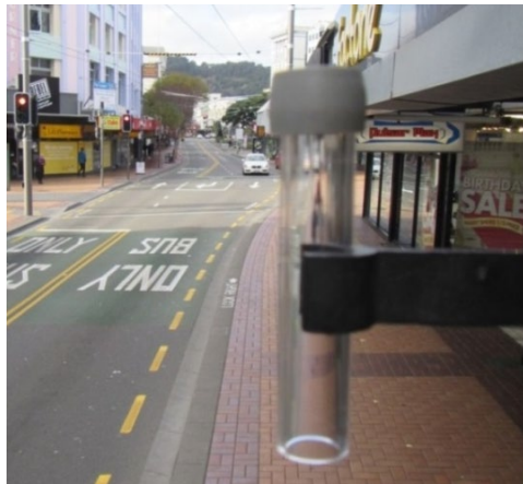
Figure 3.1: Passive NO 2 diffusion tube installed on Manners Street (WEL082)
