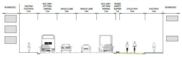
Figure 6: Proposed Thorndon Quay Cross Section
