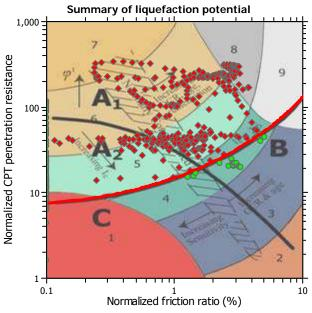
Zone  $A_1$ : Cyclic liquefaction likely depending on size and duration of cyclic loading Zone  $A_2$ : Cyclic liquefaction and strength loss likely depending on loading and ground geometry
